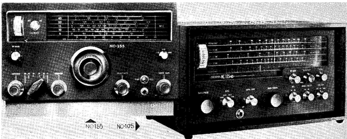
On the left, the new (American) National NC-155, an amateur-band double conversion superhet with full spreading over the bands 80-6 metres (3.5 to 50 mc); variable IF selectivity from 0.6-5.0 kc; a sensitivity claimed to be better than 1 \mu V for a 10 dB signal-noise ratio; and what is described as "planetary 60:1 tuning." For SSB reception, there is a separate product detector, sideband AGC, and a BFO calibrated for USB/LSB. Other features are band-edge calibration, automatic noise limiter and an edge-reading S-meter which follows on all reception modes. The receiver on the right is the National NC-105, a general-coverage design in the same category, having a frequency range of 550 kc to 30 mc in four bands. It also has a Q-multiplier, a product detector and a series gate type noise limiter. Calibration charts are supplied for the amateur and broadcast short-wave bands.
