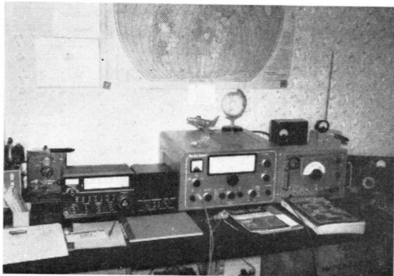
G3OSH is operated by Arthur Haines, at The Laurels, Roping Path, Yeovil, Somerset. The SSB side of the station (left), consists of a Drake 2B receiver and K.W. Viceroy Mk.III, auxiliary items including an F/S meter, ATU, crystal calibrator and a home-built Top Band Tx. On the right (featured with G3OSH himself) are a home-built NBFM transmitter for 20-40-80 metres and an Eddy-stone 840A receiver. Aerials include a Minibeam, various doublets and a long-wire for the LF bands. G3OSH first became interested in "wireless" (as we knew it then) in 1922, obtained an artificial aerial licence in 1929, and the present call sign in 1960. He says he is "Essentially a communicator, ready to work all and sundry on any band, and is naive enough to enjoy QSL'ing."
